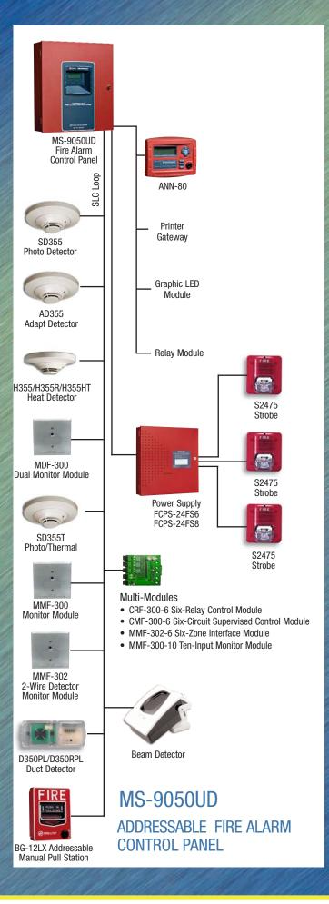
modules, and, is especially beneficial when retrofitting existing devices. The new annunciator bus provides connection for a total of 8 remote devices such as 80-character LCD annunciators for remote display of system status and control of drill, acknowledge and silence functions as well as remote printers, relays and graphic annunciators.
